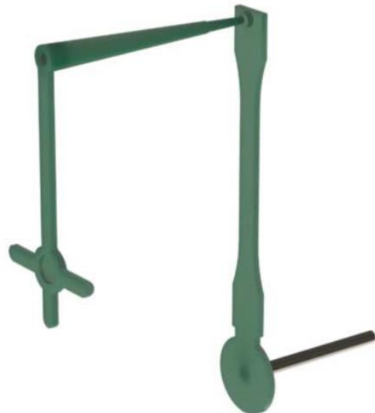
1. Figure: Injection moulding specimen and channel remainder
