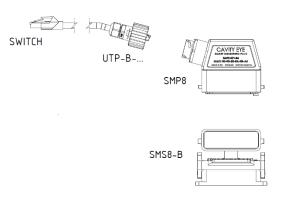
e) Connect the SCP device tot he SCS socket ont he machine, and then fix securing clip.
